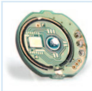
**Piezo-resistive silicon measuring cells**
